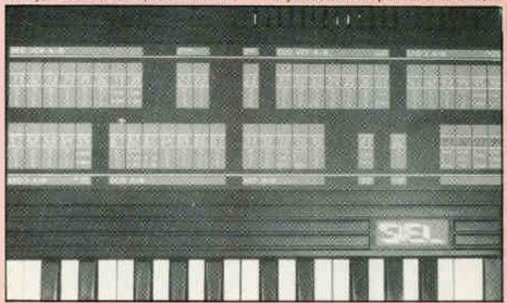
Release phases, all variable between values of 00 to 15. Nice to see Siel adopting Break Point (the level at which the Decay halts) and Slope (the rate at which the contour moves from Break Point to the Sustain level), because both make useful extensions to amount of control you have over the way the sound changes through time.
